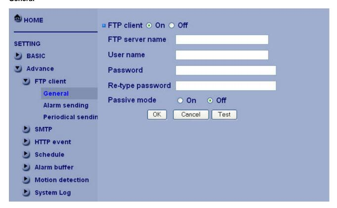
FTP client function: To activate the FTP client function, select On. The FTP client setting page appears. When you do not wish to use the FTP client function, select Off.
